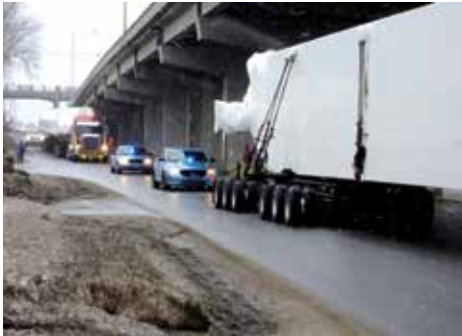
1. The first, or East Crane, so-called because of its installation location, arrived in Bath as two girders on two trucks with a state police escort every mile of the journey. Here, the first truck begins to turn.
